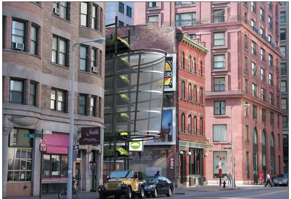
This design by Boston-based Moskow Architects for a Zipcar Dispenser in the city, which would stack cars in mechanisms above unused alleys while employing the machinery's scrim-like designed surface for advertising, is one of six winners the Boston Society of Architects' Unbuilt Architecture Design Award.
